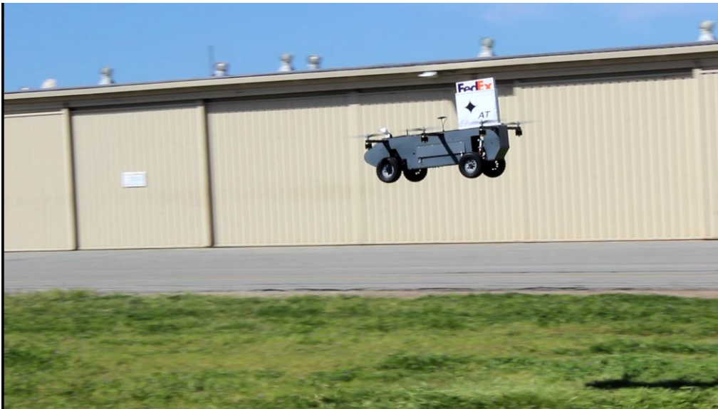
Figure 5: AT Panther in package delivery in flight testing
