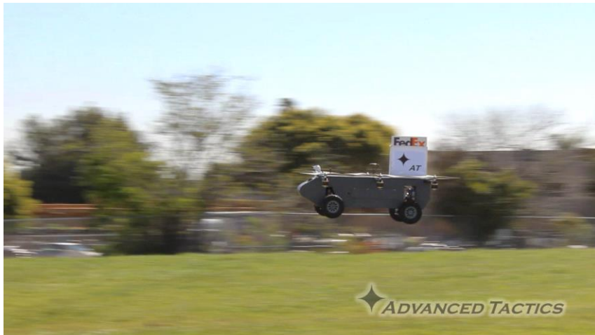
Figure 9: The AT Panther VTOL Air/Ground Robot shown during high speed fly by with package
