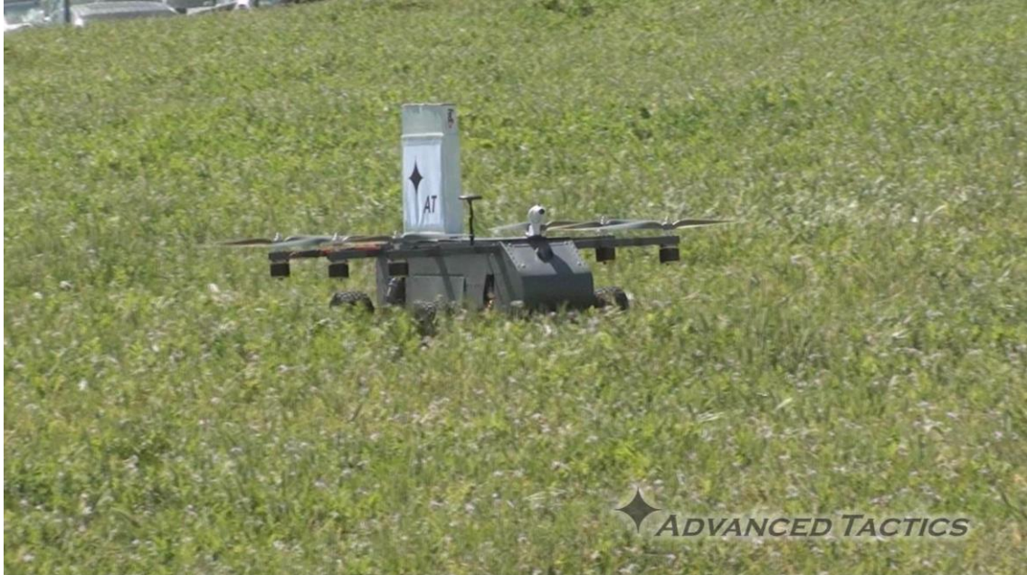
Figure 2: As seen in the now publicly released video the AT Panther Air/Ground Robot can land in remote locations with varying terrains that would be considered safe for UAV operations and then drive to congested areas to delivery packages to the door step of customers autonomously or with an operator at the controls while seeing through First Person Video (FPV) Goggles.
